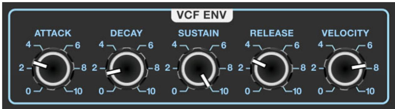
**Attack**- Defines the length of time for voltage to rise from 0V to 5V when a key is played.
