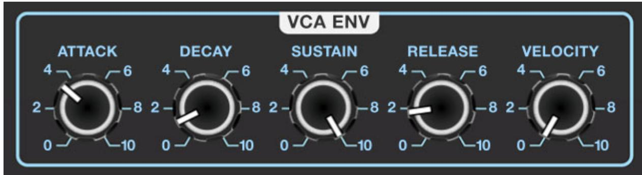
The VCA section consists of an envelope generator for control of amplitude - in other words, the "shape" of a sounds volume over time.
