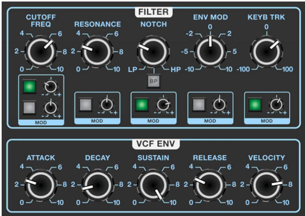
Dreamsynth uses a 12 dB/oct state-variable filter. "State-variable" refers to its curves - its Notch knob lets you choose lowpass, highpass or anywhere in between. The BP button bypasses the Notch knob and enables bandpass mode. The 12 dB/oct curve gives it a brighter overall tonality than a typical ladder filter, which works well with Dreamsynth's many brighter, bell-like digital waves.
